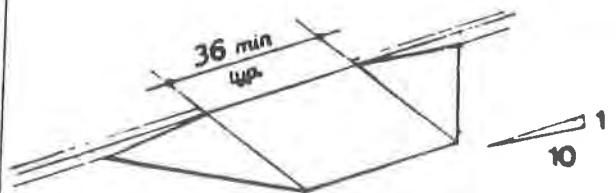
Fig. 13 Built-Up Curb Ramp
